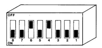
EXAMPLE: If you have a disk controller in slot 6 and a modem in slot 4, you should now have switches 4 and 6 OFF and all the other switches ON.
